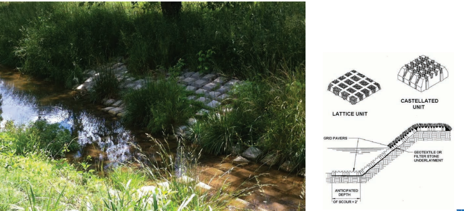
Figure 2.3.18 (Left) Example Streambank Stabilization Option 2 - Pre-Cast Revetment Grid (Sample Photo: Courtesy of Submar, Inc.). (Right) Typical Pre-Cast Revetment Grid. (Courtesy of PA Department of Environmental Protection, Best Management Practices)
